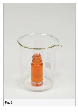
Fill water into the beaker without pouring it on the oil. As soon as the water level reaches the height of the mouth of the bottle, add the water very slowly and only at the edge of the beaker (Fig. 4). Stop the addition when the water level is about 3 cm above the mouth of the bottle (Fig. 5). Slowly put a little detergent on the water surface above the mouth of the bottle.
